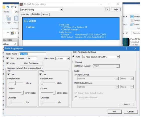
The radio name is what the remote control program on the REMOTE PC will see will see when LOCAL and REMOTE PCs are connected. Set all other settings as shown. If the auto Com port setting does not reflect the port from the Windows device manager, it can be set manually.
