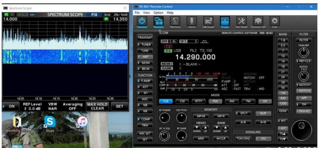
If you don't get the scope to start, the most common error is that you have not set the communications speed to 115200 Baud in the IC-7300 yet.
