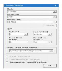
If the "Connect Setting" box is greyed out as shown above - it means the program is trying to connect and therefore will not let you change the settings. Follow the steps below.
