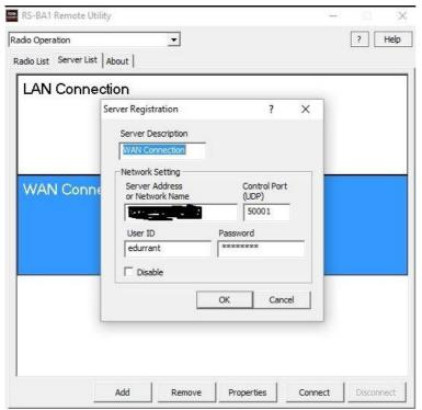
The blacked out field will contain either your Internet static IP address if you have one or the domian name of your domain defined on a Dynamic DNS service provider such as DYNDNS or NOIP. The control port will need to change only if you have had to change the ports in use in
