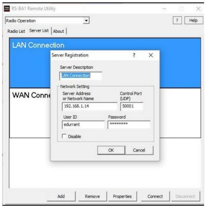
and now also through the same (radio operation/server list) panel – we configure the connection to be used when you are away from home and connecting from an Internet Cafe or via a 3G data connection, into the Internet and then on into the LOCAL PC at home:
